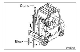
② While supporting lift chains, remove the split pins and slide out chain anchor pins from the chain anchors of stationary upright.
