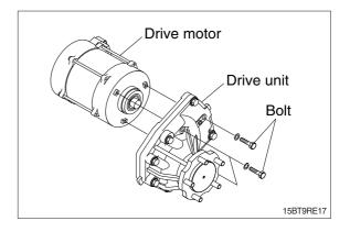
④ Loosen seven mounting bolts on the truck frame and carefully take out the drive unit.
